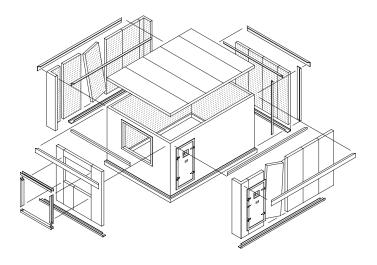
Pre-formed corner panel reduces field labor while increasing overall unit strength.
