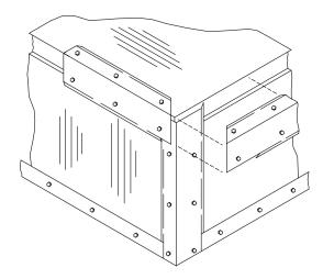
Roof trim easily connects wall panels to the roof with self-tapping sheet metal screws at the roof panel joints and internal channels.
