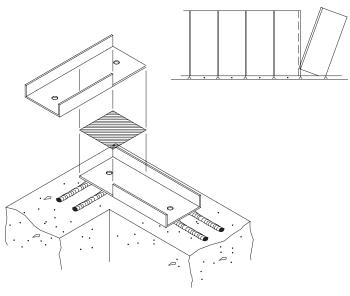
Panels are slipped into the base channel and secured with self-tapping sheet metal screws at the base channel to maintain plumb - screws at the joints are NOT required.
